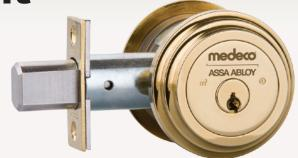
Deadbolt is available as a single- or double-cylinder or with a unique "captive thumbturn." The captive thumbturn converts the inside cylinder to a thumbturn for safe exit when the facility is occupied. A quick conversion when the facility is not occupied returns it to double cylinder mode and guards against unauthorized entry or exit. Maxum® deadbolts offer maximum protection with solid-brass construction, along with anti-drilling and anti-prying features.
